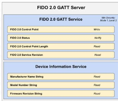
**Figure 5** Mandatory GATT services and characteristics that **MUST** be offered by a FIDO Authenticator. Note that the Generic Access Profile Service ([BTGAS](#)) is not present as it is already mandatory for any Bluetooth Low Energy Technology compliant device.
