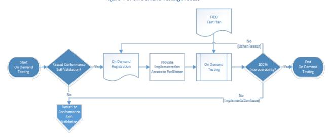
Figure 4-3: On Demand Testing Process
