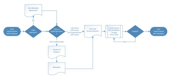
Figure 3-1: Conformance Self-Validation Process
